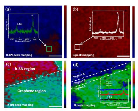
FIG. 3. Raman mapping of Sample B for (a) h-BN  $E_{2g}$  peak of h-BN, and (b) graphene G peak at one surface area, and (c) h-BN  $E_{2g}$  peak and (d) graphene G peak at another surface area. Insets show Raman spectra accordingly. All scale bars are 1  $\mu$ m.
