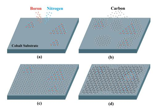
FIG. 4. Schematic of growth mechanism for the MBE growth of h-BN/graphene heterostructure on Co substrate. (a) h-BN nucleation on Co substrate, (b) initial graphene nucleation on Co substrate and edges of h-BN flakes, (c) lateral growth of graphene, and (d) layer-by-layer graphene growth on graphene and lateral graphene growth on h-BN flakes.
